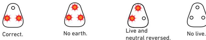
If any of the Surge Safe Plug lights are **ON** when the wall socket switch is **OFF**, then switch **ON** the wall socket switch and the following applies:
